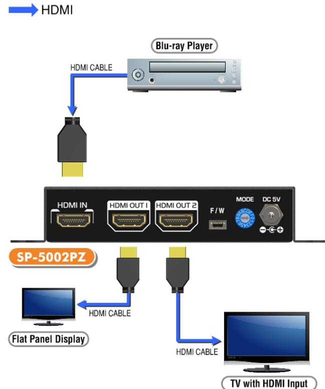
1. While connecting a new monitor to the splitter under mode D (auto EDID) & mode E and F (EDID learning), experiencing a short period of time without displaying might be expected. The splitter will do Automatic EDID learning which analyzes the newly connected monitor to see if the EDID for the HDMI input is necessary to update!
